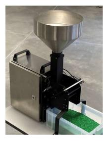
litres), the SPECTRO-3-0°/45°-MSM-LAB-DIG-LF color measurement system can be used. This system also uses a sight glass, so that the same measurement setup is used as for inline applications.
