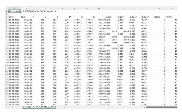
EXCEL® file with the L\*a\*b\* and the dL\*, da\*, db\* and dE values, the tristimulus values X, Y and Z, and the time and date.
