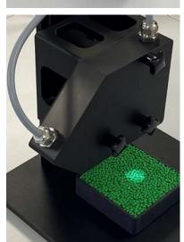
If only a small amount of recyclate is available for laboratory-based color measurement, it can be performed using the compact SPECTRO-3-0°/45°-MSM-CMU using only 0.15 litres of recyclate. The measurement is performed through a sight glass and corresponds exactly with the method used on the inline systems if a sight glass is required at the site of use. If on the other hand, sufficient recyclate is available for color measurement (up to 10
